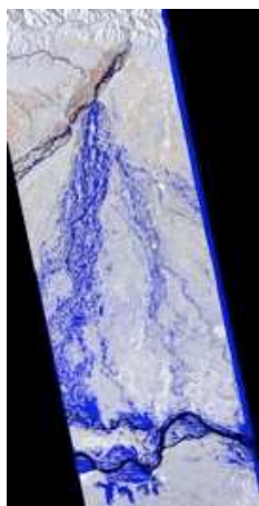
Fig. 4. Multitemporal composition obtained automatically in FAIRE and used to support image analyst in generating flood maps. The image is related the flood that affected Bihar State, India, in August 2008. Blue colour represents the areas most likely flooded. The image analyst has to further interpret such image determining which areas are really flooded and avoiding false alarms (due for example to other kind of changes).
