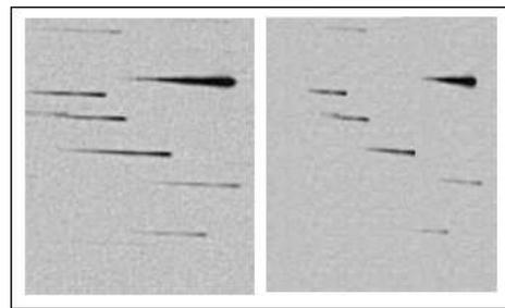
**Fig. 6.** Left: Part of digitised Byurakan Sky Survey plate (spectral resolution 10 nm/mm at  $H\gamma$ ), Right: Re-scaling to simulate the Gaia BR/RP resolution (18 nm/mm at  $H\gamma$ ) This is a part of the efforts to develop an alternative and real Gaia BP/RP simulator.
