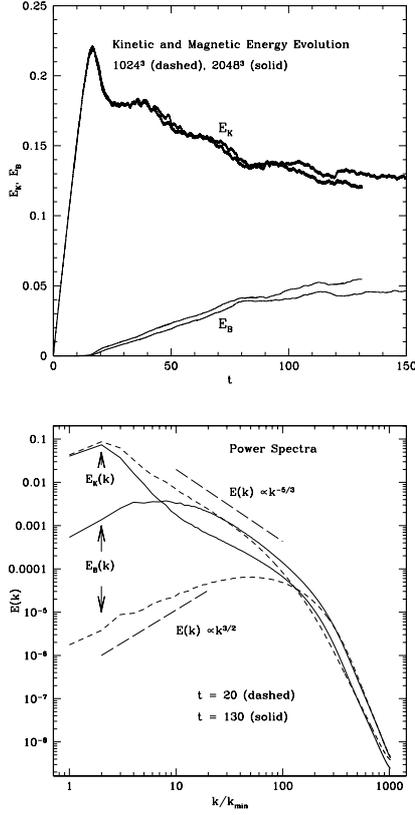
**Fig. 1.** Top: Evolution of kinetic,  $E_K$ , and magnetic,  $E_B$ , energies in simulations of ideal, compressible MHD turbulence for two grid resolutions. Bottom: Power spectra,  $E(k)$ , of kinetic and magnetic energies at  $t = 20$  and  $t = 130$  in the  $2048^3$  zone turbulence.
