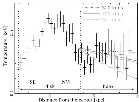
**Fig. 5.** Observed temperature profile obtained from the hardness ratio profile in the SB region. The expected temperature profiles with constant velocities of  $300 \text{ km s}^{-1}$  (dot),  $100 \text{ km s}^{-1}$  (solid) and  $50 \text{ km s}^{-1}$  (dot-dash) are also plotted together. Dashed line exhibits the observed steepest temperature slope within the 90% confidence level.
