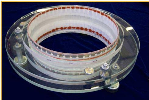
**Fig. 1.** The first prototype shell of thin glass assembled. The focal length is 5500 mm. The diameter at intersection plane is 487 mm. The glass thickness is 2 mm. The total length is 200 mm. The mirror optical profile is polynomial. It is made of fused silica and weights is 1.37 kg.
