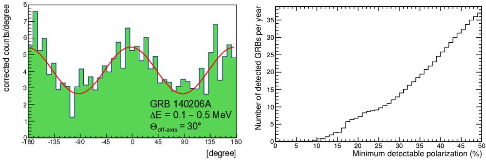
**Fig. 3.** *Left panel* – All-Sky-ASTROGAM polarization response in the 100–500 keV band to a GRB like GRB 140206A ( $z = 2.739$ , see Götz et al. 2014) detected at  $30^\circ$  off-axis, assuming a polarization fraction of 75%. *Right panel* – Cumulative number of GRBs to be detected by All-Sky-ASTROGAM as a function of the MDP at the 99% confidence level.
